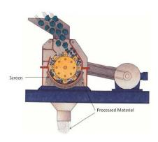
In any given size reduction application, the specific properties of the material being processed play a key role in how the desired finished particle size is achieved.
